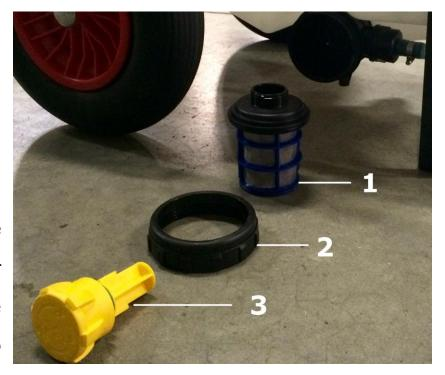
Accommodate filter on his carcass, screw threaded ring, push and turn right  $\frac{1}{4}$  round the unlocks quick release system to lock him.
